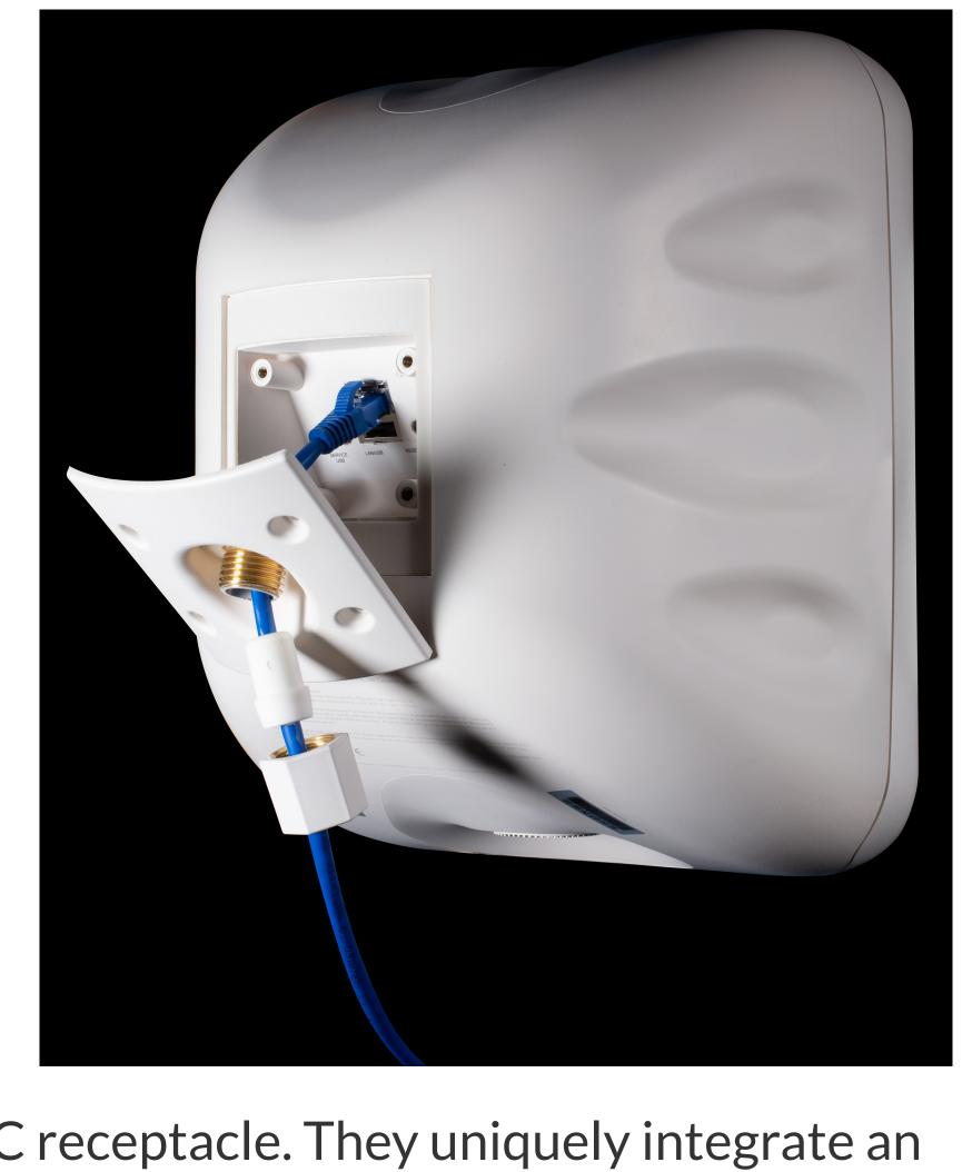
in-built streamer and amplifier for an all-in-one solution. Thus, opting to use PoE speakers significantly reduces the amount of hardware required since you don't need to purchase a separate amplifier or streamer, you don't need two different connections for network and power, and best of all, you don't need to worry about placing them near or spending a fortune on providing AC receptacles.
